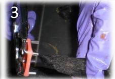
Close the handles of the elastrator to open the pins to their full capacity to open/stretch the rubber ring.
